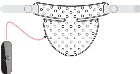
Connect the remote control to the mask using the USB-C cable. Connect the second cable to the DC port on the remote for charging.
